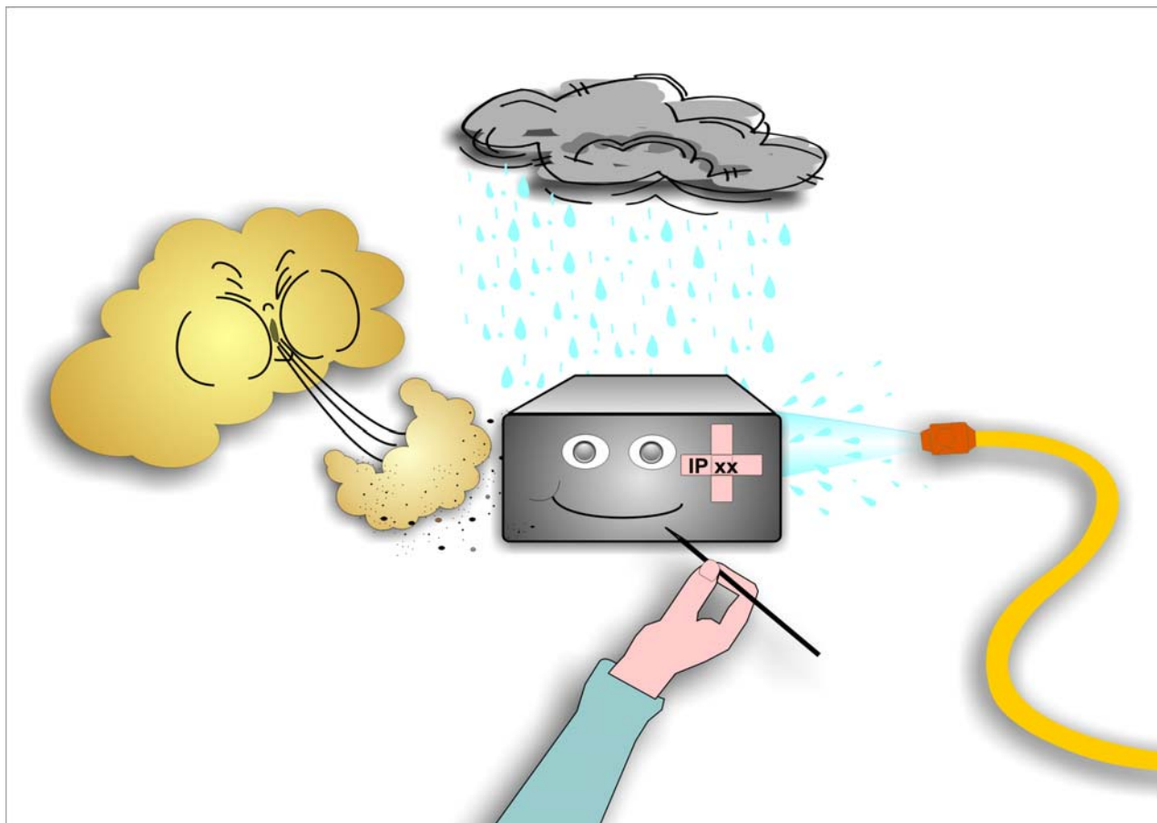
Fig. 25: IP factor – Protection by enclosure
